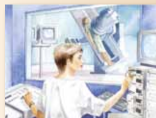
A large surface control window made from radiation shielding glass enables the technician to monitor the X-ray process.
